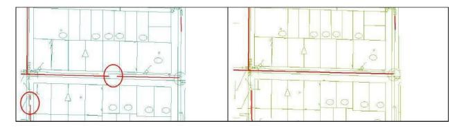
The short pipe that connects pipes (for example, pipes in the fitting, pipes for fire hydrants, etc.) should be drawn separately but connected to pipe assets
