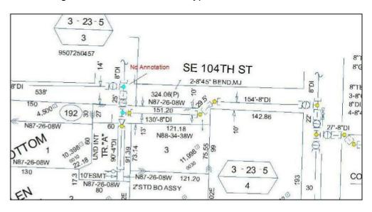
Example of Reading Difficulty of Annotation- There is no way to tell which annotation is connected to which drawing. So, all annotations should be in proper location to understand attributes clearly.
