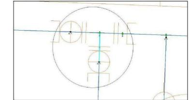
Pipe (long and short) shall not be broken by other assets outline or periphery; it needs to be continuous line and break must be based on the center points of the connecting assets not on the circumference or periphery
